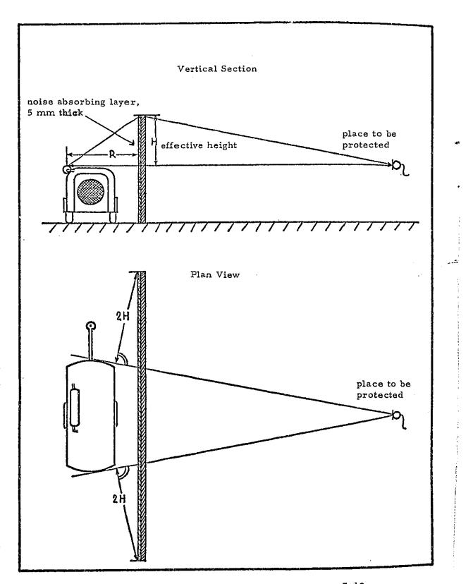
Figure 7-2. Noise shield for construction machine 7-19
